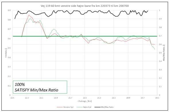
Figure 14 - Surface quality using friction data on Vej 119
