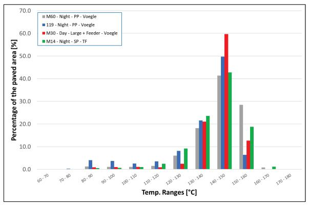
Figure 11 – Temperature distribution of the paved KVS sections
