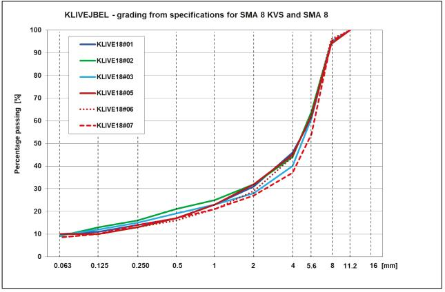
Figure 1 - Grading curves from the asphalt contractors' specifications
