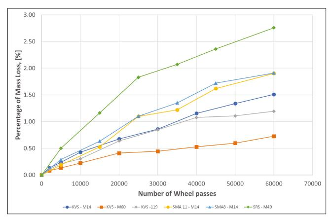
Figure 8 – Wear data calculated as percentage of mass loss
