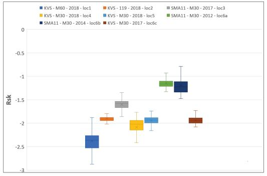
Figure 20 – Skewness data measured on M30, M60 and 119.
